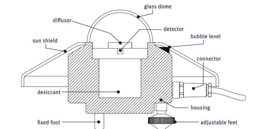
The SUV5 has a sealed construction with a non-replaceable internal drying cartridge. The internal desiccant lasts for 10 years.
