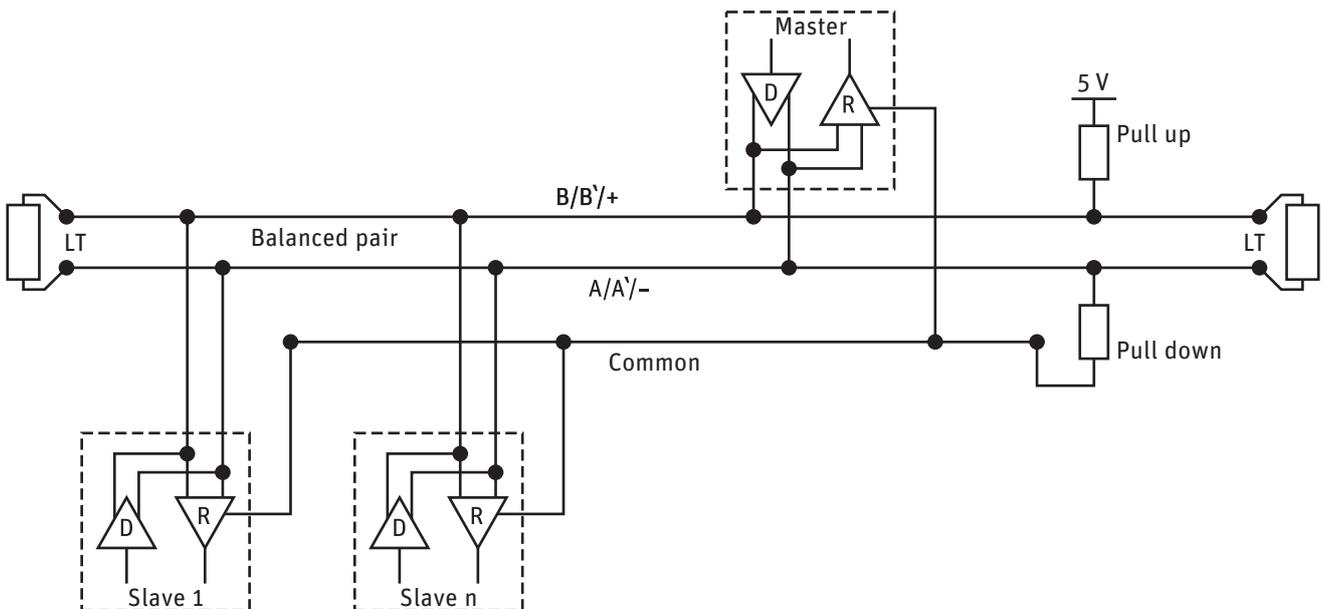
The slaves may be a SUV5 radiometer or any other Modbus® devices. If a SUV5 radiometer is the last device on the network a line terminator (LT), consisting of a 120 Ω or 150 Ω resistor, must be connected between terminals A/A -/ and B/B +/. Never place this line termination on the derivation cable. It is also required to install the pull up and pull down resistors as shown. The value of these resistors must be between 650 Ω and 850 Ω.
