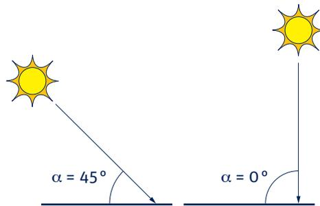
Ideally a radiometer has a directional response which is exactly the same as the cosine-law. However, in a radiometer the directional response is influenced by the detector and by the quality, dimensions and construction of the dome(s). The maximum deviation from the ideal cosine-response of the radiometer is given up to  $80^\circ$  angle of incidence with respect to  $1000 \text{ W/m}^2$  irradiance at normal incidence ( $0^\circ$  zenith angle).
