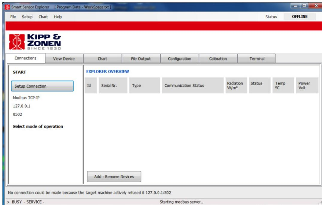
To connect a smart radiometer to a PC, a RS-485 to USB converter is required. Recommended is using an isolated version like the 'USOPTL4' from B&B for safety and protection of the PC.
