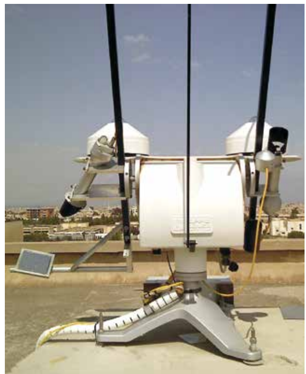
A TraCS system measures the soiling effects on mirror reflectivity in real-time
